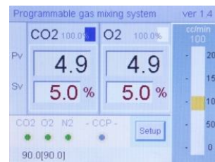
Tri-gas control & flow meter
